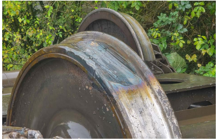
The damaged wheel thought to have been the cause of the incident. Photo: Rail Accident Investigation Branch
