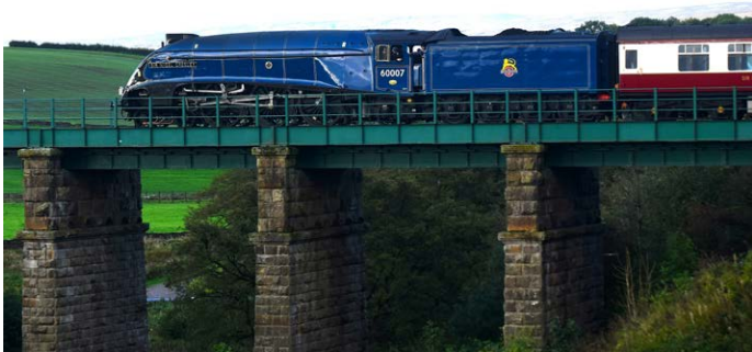
LNER Class A4 4-6-2 locomotive, no 60007 Sir Nigel Gresley – the 100th “Pacific” locomotive that had been designed by the great engineer and thus named after him - crosses Clapham Viaduct on 21st September. Photo: Andy Scott
